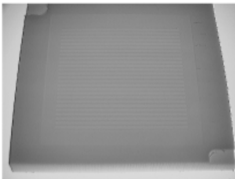
[Step 4] Mold cut by Ball Endmil
